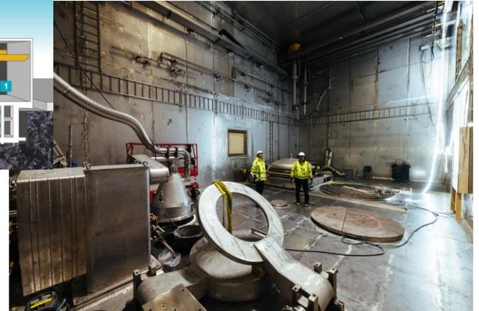
Docking stations for the canister and the fuel transport cask, drying station for spent fuel at the fuel handling cell
